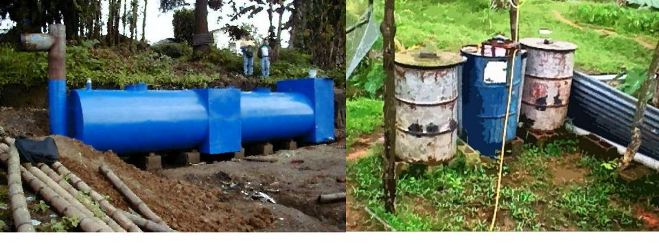
The most effective biodigester design is the Up-flow Anaerobic Sludge Blanket, with a double wall for circulation of waste steam or hot water to increase temperature.
