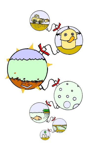
The anaerobic digestion of the 'waste' is followed by a **sedimentation process**, where heavier material is allowed to precipitate allowing water infused with other lighter materials and organisms to flow to the oxidation basins and ponds.
